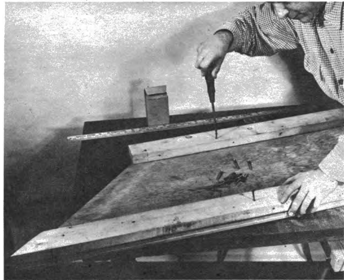
FRAMING of 2-by-3's is fastened with 1\frac{1}{4} -inch screws to sides, \frac{3}{4} -inch in from edges, to permit recessed front, back panels.
